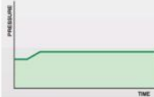
Pressure increased based on degree of flattening. Flow limitation produces a fine adjustment
